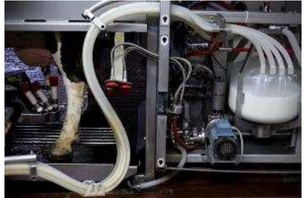
After luring the cow with sweetened pellets, charting the cow's weight, scanning and cleaning its teats, the automatic milking system milks a cow on the Groetsch family farm in Albany, Minn.
